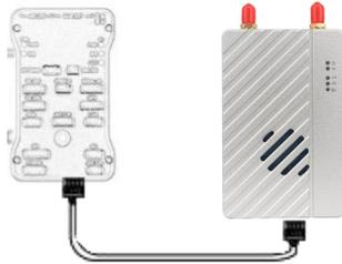
2. Connect the RC receiver to the ground unit
