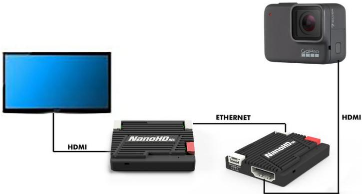
As shown, connect the HDMI port of the camera to the NanoHD N1 HDMI interface, and connect the HDMI interface of NanoHD N6 to the display. Connect the NanoHD N1 to the NanoHD N6 through the custom network cable in the accessory box.
