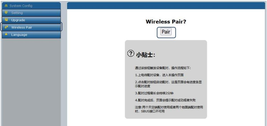
The Wireless Pair function is used to pair the air and the ground. The operation process is as follows: Power on the device. Click " Pair "button to start pairing, and there will be a progress bar to show the pairing progress; The pairing process lasts up to 2 minutes; When the pairing is complete, the page will display a message indicating that the pairing succeeded or failed. The signal strength indicator light will indicate the current pairing state in the form of a water lamp.
