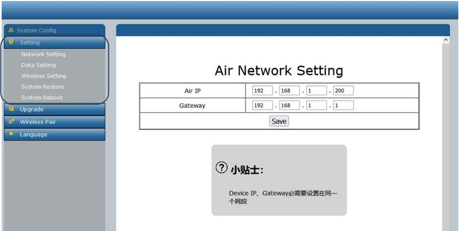
Air Network Setting can set the Air IP address and gateway address. The following table describes the parameter values. The Device IP address and Gateway must be on the same network segment.
