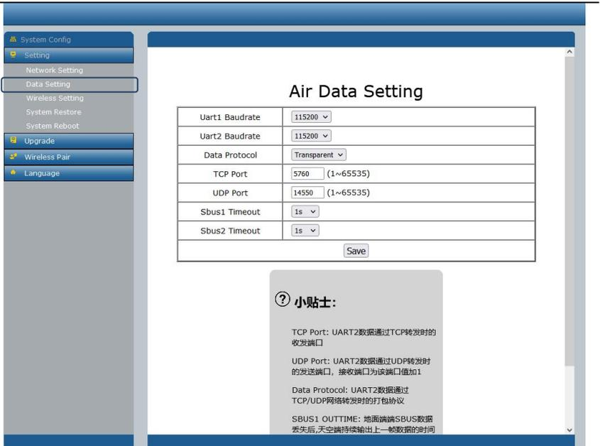
The Air Data setting can set the baud rate of the serial port on the air, the packet protocol for data transfer from serial port 2 to network forwarding, the TCP/UDP port number for network forwarding, and the output timeout period after SBUS data lost. The following table describes the parameter values.
