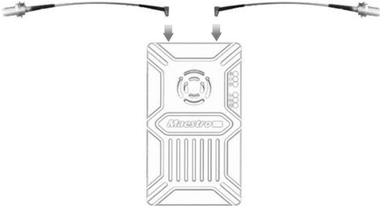
1.2 Fixed the device and RF cable on your drone. Install the antenna. Pay attention to the connection of the antenna to tighten. Make the antenna downward. There is no metal or shielding within 20cm of the antenna.
