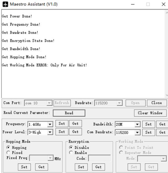
After step1, click 'Read' button. All current parameter will print on the information display. Because the Working mode is only for air unit. The Working mode box will turn grey on ground unit configuration.
