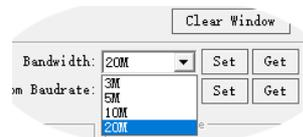
data can be transmitted, but the weaker the anti-interference. In Fixed frequency mode, M50/M51 will have more frequency to fix with small BW.
